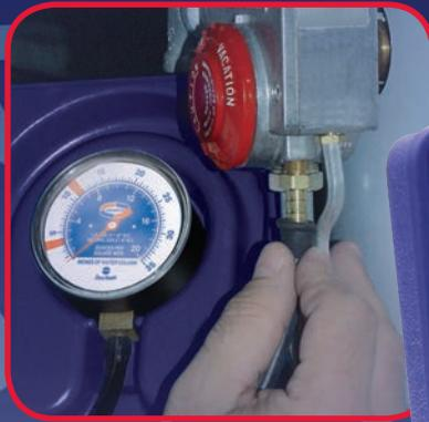
A new Uniweld design feature allows you to easily zero reset the gauge needle by simply twisting open the dial lens to access the adjusting screw located on the dial face.
