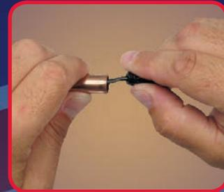
The 70079 Inside/Outside Deburring Tool removes burrs and sharp edges with double edge steel blades. This heavy duty metal deburrer has a capacity of  $\frac{1}{8}$ " to  $1\frac{5}{8}$ " O.D. (3mm to 42mm).
