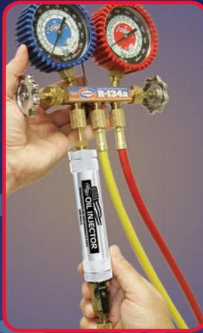
The refillable Oil/Dye Injector has a 2 oz. capacity. The anodized aluminum body and end caps are fitted with O-ring seals. Attach the injector directly to the manifold low side hose connection and add oil/dye to the system. Available with optional 1/2" ACME fittings or 1/4" Flare fittings.
