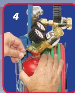
**[STEP 4]** When you have completed the job and are ready to shut off the torch, **always shut the oxygen valve first and then the fuel gas valve [acetylene]**. **NOTE:** Shutting off the fuel gas first can cause backfire and/or flashback.
