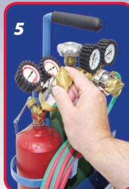
**[STEP 5]** To shut down the torch for storage or transportation, close the cylinder valves. Release the oxygen pressure by opening the oxygen torch valve [vent safely]. Close the torch valve and repeat this same process for the fuel gas [vent safely]. Close all valves tightly and secure the equipment. **Now the shutdown is complete!**
