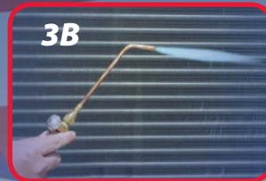
Next, open the oxygen and adjust the flow until the white feathers disappear into a well-defined bullet nose cone called the neutral flame [3B].
