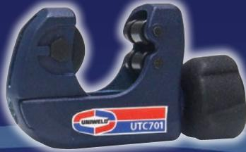
The Mini Cutter rollers are grooved to allow close cutting at flared end of tubing.
