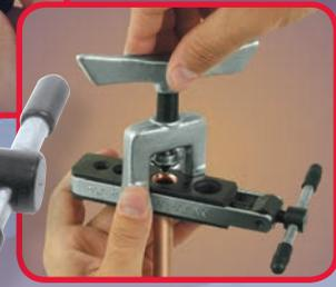
For 45° flaring of 3/16", 1/4", 5/16", 3/8", 1/2" and 5/8" O.D. soft copper, aluminum and brass tubing.
