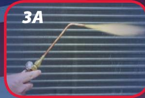
**[STEP 3]** To light the tip, **open the fuel gas [acetylene] valve first about 1/2 turn** and quickly ignite with a spark lighter. Adjust the flame so that it is not separated from the tip end. The flame should be bright yellow with no black soot [3A]. If necessary, increase the fuel to clear the black soot.
