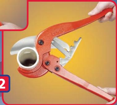
2 Position pipe in the cutter and close handles together to engage ratchet. Blade begins to cut on contact.
