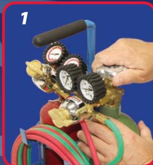
**[STEP 2]** After the proper tip has been selected and installed, the proper operating pressure needs to be determined from the manufacturer's tip chart. Set each regulator's corresponding pressure by adjusting the pressure adjusting screw. Purge hoses and equipment by briefly opening and closing the oxygen valve and fuel gas valve separately and venting gases safely. Purge hoses and equipment before each use.
